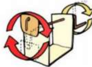
a simple crank mechanism for chewing the head (not shown) is fixed, the lower jaw moves
